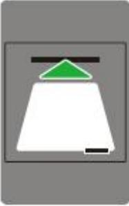
A diagram of a grey ID card reader. A white ID card is partially inserted. A green triangle points downwards from the bottom edge of the card, indicating the magnetic stripe is facing down. A black horizontal line is visible below the card's bottom edge. | <p>Installation position: track facing down</p> <p>Insert the ID card into the ID card reader as shown in the picture.</p> |
