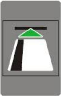
A diagram of a grey ID card reader. A white ID card is partially inserted. A green triangle points upwards from the top edge of the card, indicating the magnetic stripe is facing up. A black horizontal line is visible above the card's top edge.            | <p>Installation position: track facing up</p> <p>Insert the ID card into the ID card reader as shown in the picture.</p>   |
